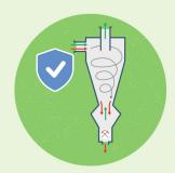
Controlling dust from wood substitute materials production processes by installing the multicyclone air purifiers and electrostatic precipitators with an 80% and 99% efficiency in dust control, respectively.
